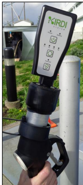
FIGURE 4-4 HHT ATTACHED TO HYDROGEN NOZZLE
