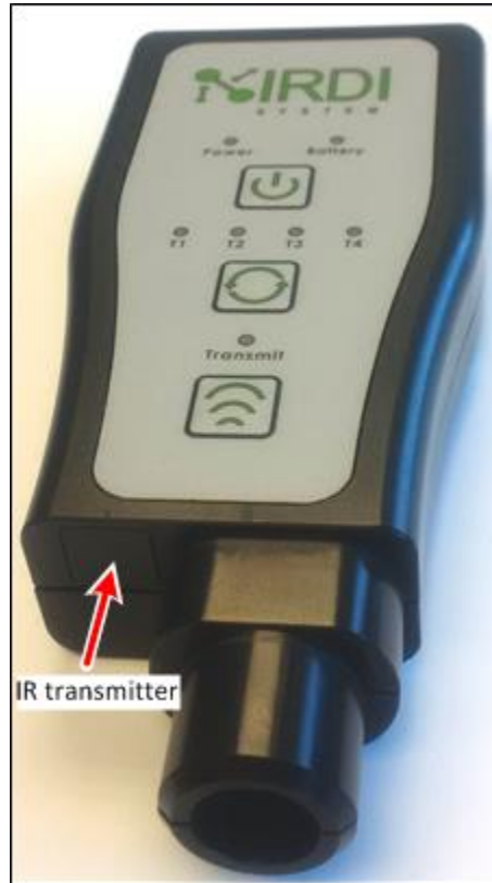
FIGURE 4-2 HHT INFRARED TRANSMITTER LOCATION
