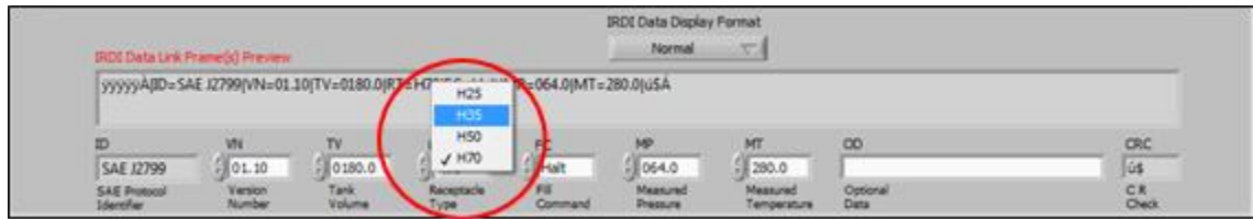
FIGURE 5-15: HHT TEST PATTERN SOFTWARE - RECEPTACLE TYPE INPUT
