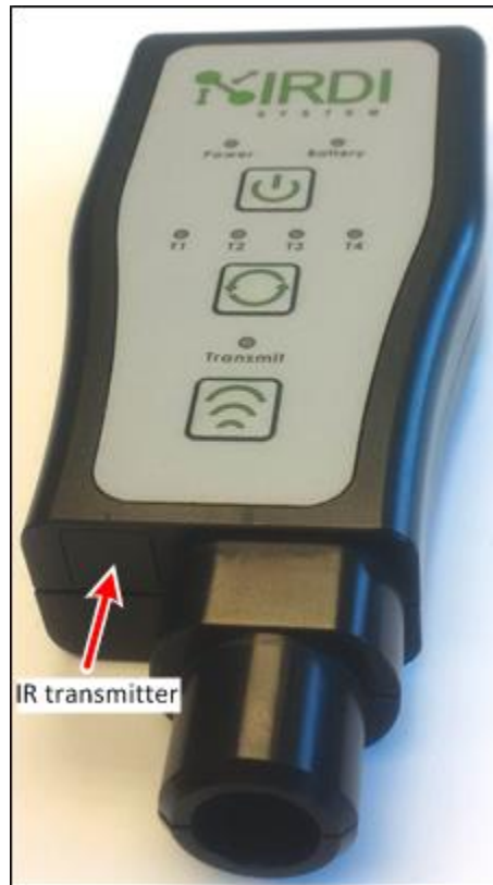
FIGURE 4-2 HHT INFRARED TRANSMITTER LOCATION
